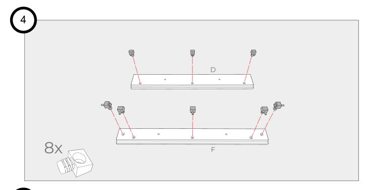
Note: We recommend dry-fitting wood panels before gluing to check the fit. Apply wood glue to channels where wood panels joint just before attaching. Repeat this for all wood joint pieces as you progress through
